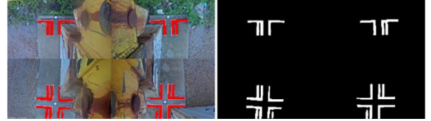
a) corner line mask map b) corner line foreground binary map Figure 7. Binary Image Of Corner Line Foreground
