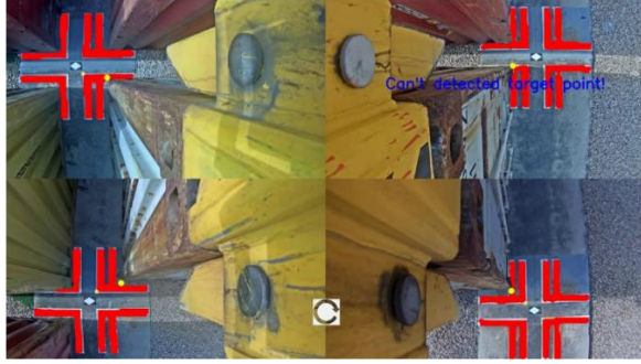
Figure 19. The Top Right Container Corner Line Blocked
