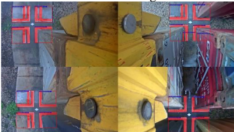
Figure 6. Container Corner Detection And Segmentation Results
