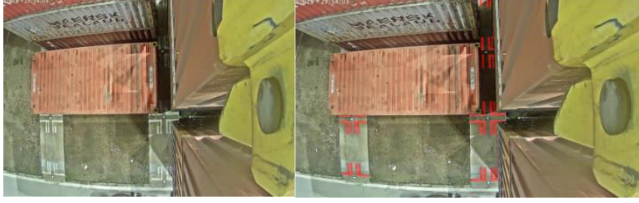
a) original image b) annotated image Figure 5. Example of Container Corner Line Data Set Annotation
